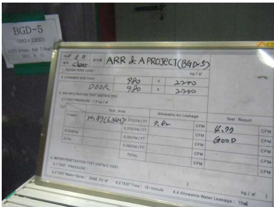
<사진> after air leakage test <BGD-5>
