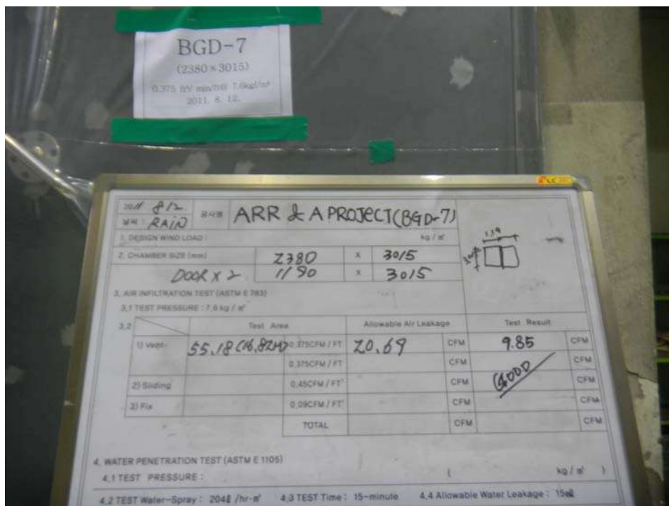
<photo> after air leakage test <BGD-7>
